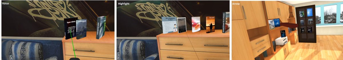
Figure 1: The three uni-directional Cross-Reality pinpointing techniques explored in the first study (from left to right): no visual feedback, audio only via voice clips; a highlight outlining the object (in white); and a three-dimensional arrow.
