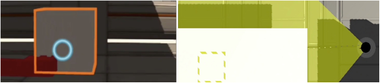
Figure 6: The highlighting technique from both the VR and tablet users’ perspectives (left and right, respectively), in response to the VR user’s head pointing (blue circle). The tablet user will perceive this even if occluded by some other element in the scene (right). Unrelated to this is a red key, which is not manipulable by the VR user in its current state (left).
