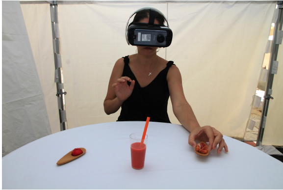
Figure 4: A user testing the full gastronomic experience. The system has been set up in a white tent, with a grey metallic structure. The three tapas can be seen from right to left: ham toast, gazpacho , and mousse. Both the food and the cocktail cutlery have high values of red chrominance, therefore appearing in the Distributed Reality blend.
