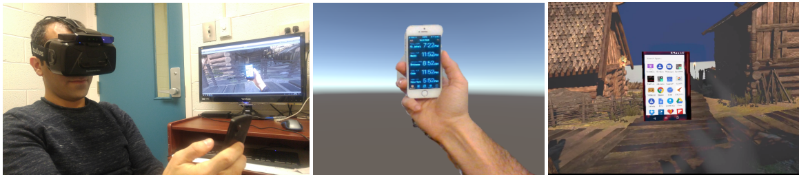
Figure 2: Near-Range Augmented Virtuality: On the left, a user holding a phone in front of the HMD. In the middle, an image of the users's hand and phone as it appears within the default virtual environment. On the right, Augmented Virtuality as it appears when using SDSC.
