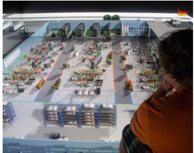
Figure 2: A user exploring a factory using the VR-based factory planning application *flapAssist* within a CAVE-like VE.
