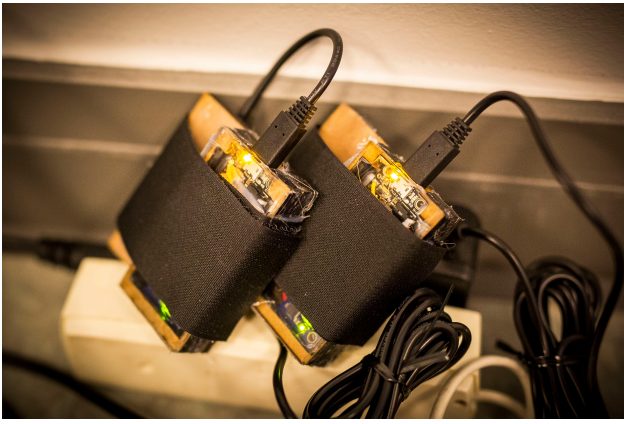
Figure 7: The tracking device with Velcro straps; here while charging the battery.
