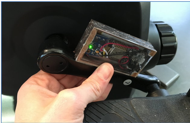
Figure 8: The mount method is on the side of the pedal arm (here without the Velcro for clearer visualization).
